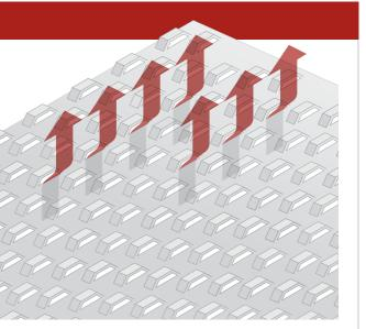
With their open area, bridge slot perforation allows permanent free flowing ventilation.
