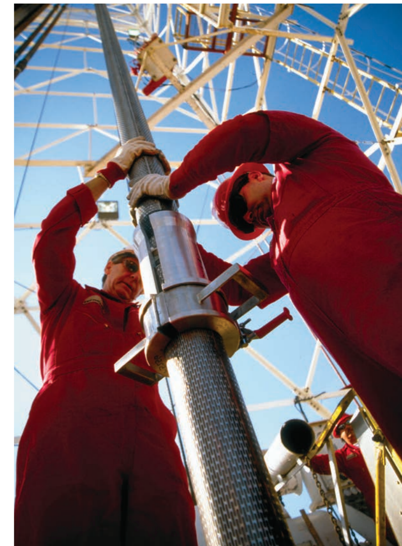
Slot hole perforation in stainless steel
